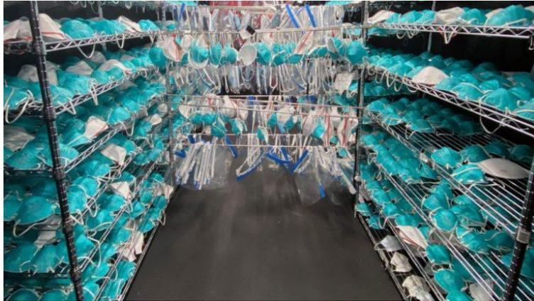
Inside the VHP chamber for PPE decontamination using Battelle's design. Image from: <https://news.stonybrook.edu/newsroom/battelle-ccds-critical-care-decontamination-system-arrives-at-stony-brook-university/>.
